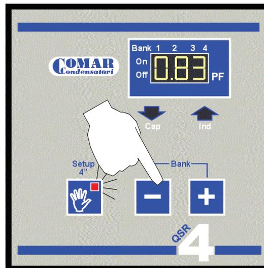
Figure 3: desinsertion batteries
