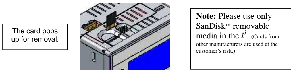
Figure 8.2 – Installing Removable Memory Card
