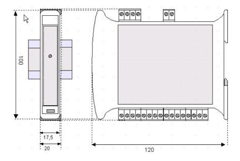
Note: Number of I/O terminal connections change with model type
