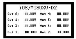
In this case, alter the output voltages and measure with a multi-meter to see that they correspond.
