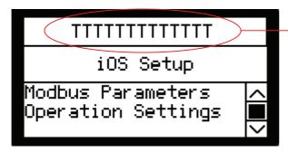
The part number of the connected unit should appear here. If it does not then comms have not been established. Try cycling power on both units, check the 'INIT' jumper and try again.
