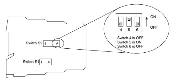
Switch S1 configures the input type and range and switch S2 configures the output type and range. The switch settings are explained on the next page.
