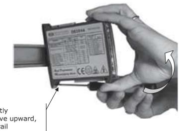
Push the screwdriver slightly downward and pull the drive upward, releasing it from the DIN rail
