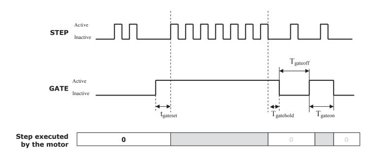
To grant a correct execution of the given commands it is necessary to respect some time relations amongst the signals. In the following table are detailed the limits to be observed.
