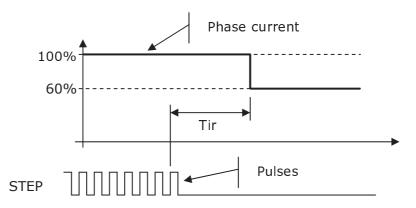
After the last STEP input disable/enable transition the *Tir* time starts to pass, after which the automatic current reduction intervenes reducing the phase current (in the example to the 60% of the nominal value, i.e. of the set configuration value).
