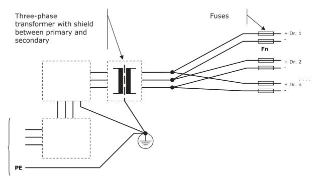
The above scheme includes a three-phase transformer (note the distribution of the drives on the three phases). If necessary it is also possible to use a mono-phase transformer.
