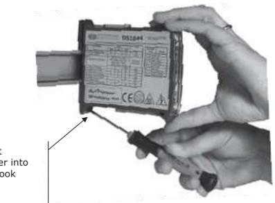
Insert a small flat bladed screwdriver into the red colored hook
