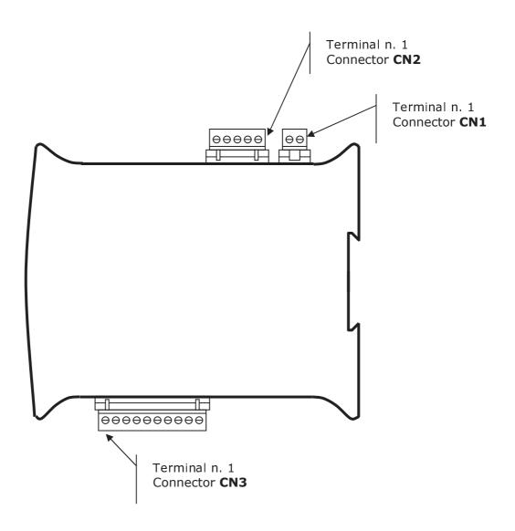
All the terminal blocks do not contain iron and are supplied with mobile truck. The clamping screw is slotted head, sized for screwdriver of 3x0.6mm.
