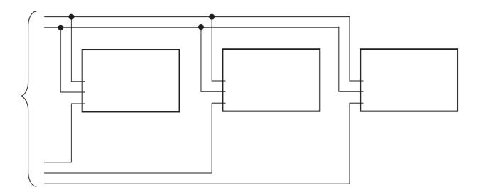
In this case the control system sends a step and direction signal to all the drives contemporaneously, while the GATE signal is activate from time to time on the only drive the control system wants to move. The drives with the GATE signal not activate ignore the pulses and maintain the motor firm.
