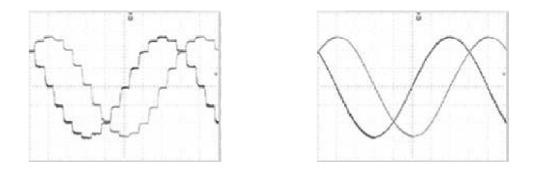
When minor resolution is working (left figure) the motor movement is noisier while when the resolution is greater (right figure) the motor moves smoothly and with less vibrations.
