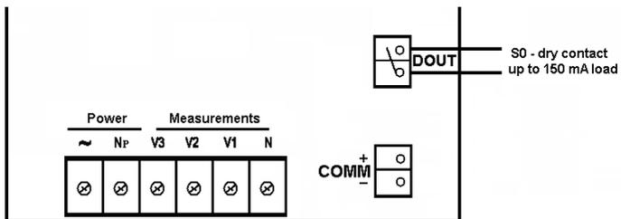
Figure 2.7 LTE 2013 Digital Out wiring example
