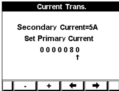
Figure 4.3 Current Transformer
