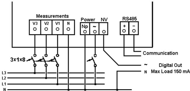
Figure 2.6 LTE Digital Out wiring example
