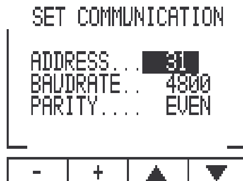
Figure 6.2 Serial Communication Setup
