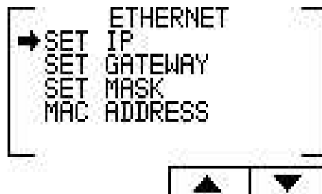
Figure 6.3 Ethernet Communication Setup
