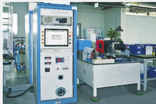
Servo Motor Testing System
