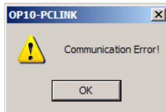
When you see the communication error, please check the power supply, whether the download cable connected in the right way and whether users have chosen the proper COM port.
