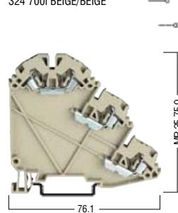
In the field of machine constructions, inductive or capacitive proximity switches are increasingly used for actuation without physical contact. In general they are designed as "Three Wire Sensors". The positive and negative conductor transmits the switching pulses ERT 3S terminal blocks minimise wiring time and costs and cabinet space when terminating three wire devices such as sensors, proximity switches etc.
