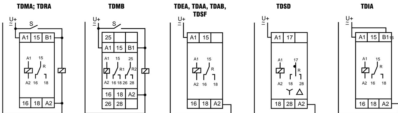
Control Function    Function Rp: without link    Function Ri: link A1-B1
