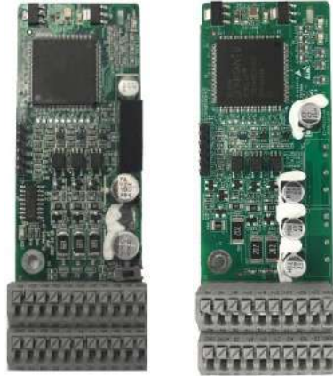
Multifunction incremental PG card HD2-E-PGIM
