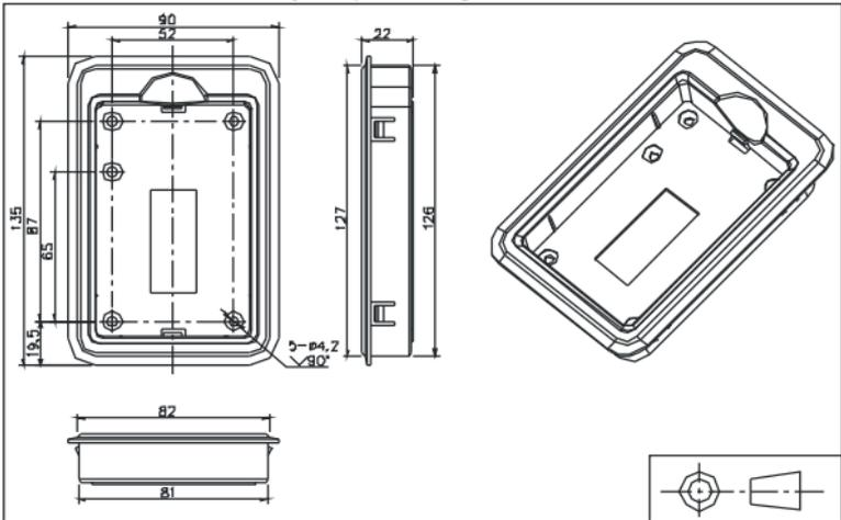
Dimension drawing of keyboard compartment (dimension unit: mm)
