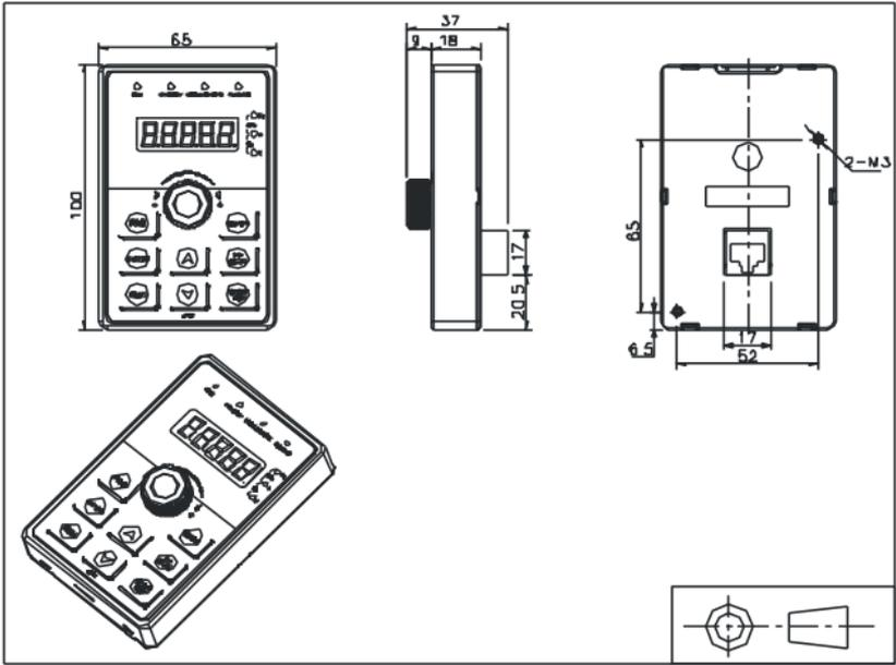
Keyboard dimension drawing (dimension unit:mm)
