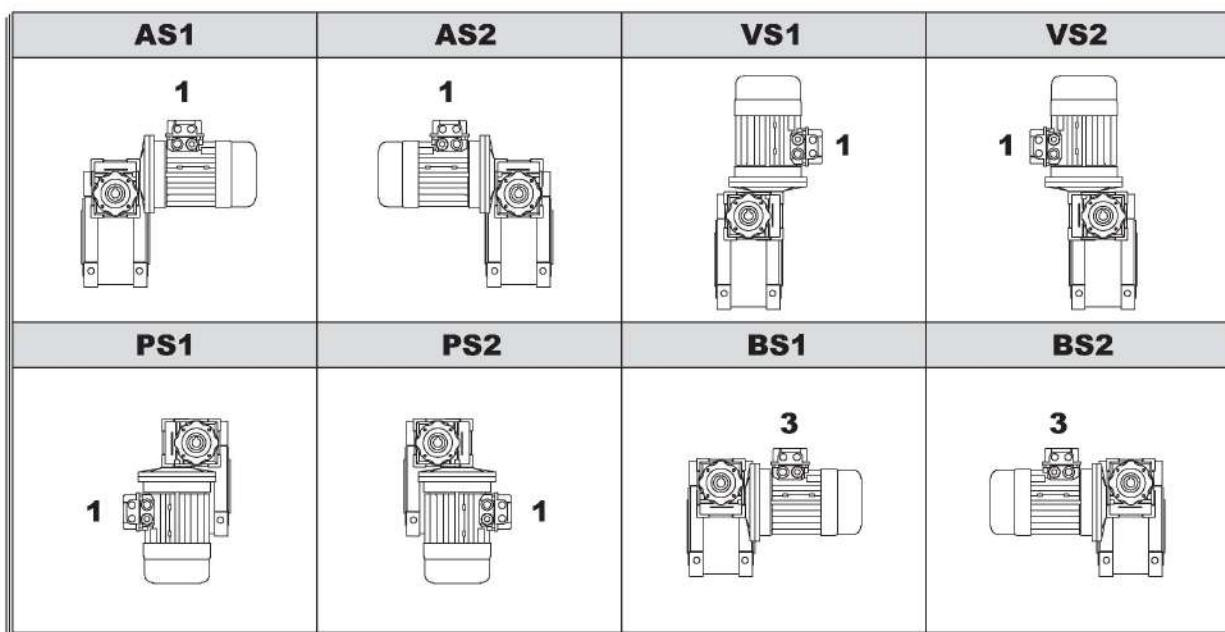
The position of the 1st reducer with respect to the 2nd gear reducer depends on the versions. Unless specified at the time of order, combination groups are supplied in version BS2. The specified mounting position refers to the 1nd gear reducer, see page 73 for the possible mounting positions.
