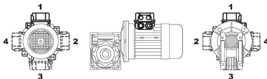
In the case of specific requirements, when ordering, specify the position of the terminal box as shown in the diagram.
