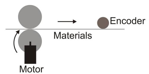
The object manages the placement of a Motor (Brushless etc..) By the encoder is made up for the slippage .
