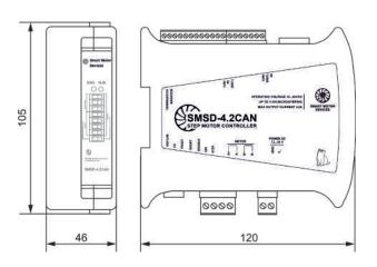
SMSD-4.2CAN is a step motor controller with CANopen communication protocol. It is designed by our engineers for medium size stepper motors. The CANopen protocol has a wide range of features for synchronization and synchronous operation of few controllers.
