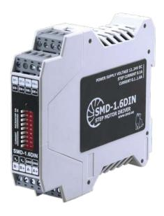
SMD-1.6DIN is a driver for small and medium size stepper motors. The driver provides smooth operation and good speed-torque performance. The driver has the STO (Safe Torque Off) function which provides motor phases deenergizing in case of any alarm situation.
