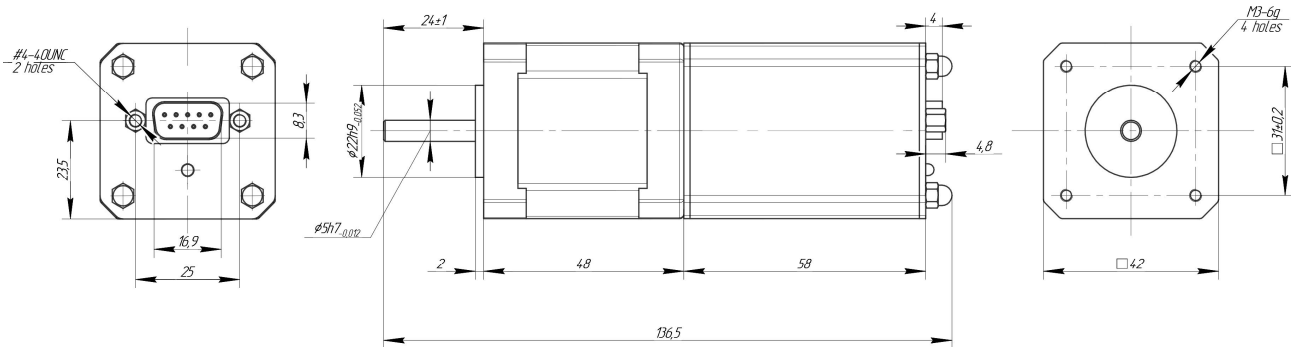
Img.4. Dimensions of stepper motor SM4247 with integrated driver SMD-1.6 mini IP65
