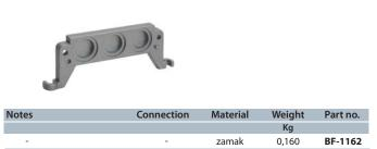
The diaphragm is not only the end plate of the manifold but it is also coupled with the exhaust regulator to separate two sub-bases and regulate the valves independently. In this case breakthe central blind hole. To get two or more pressures, break the two side blind holes.
