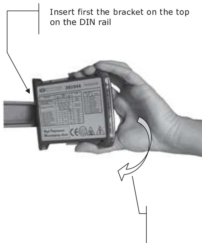
To remove the drive from the DIN rail insert a small flat bladed screwdriver into the red colored hook on the bottom, on the back of the drive. Push the hook downward and pull the drive upward slightly rotating it, releasing it from the DIN rail as shown in the picture.
