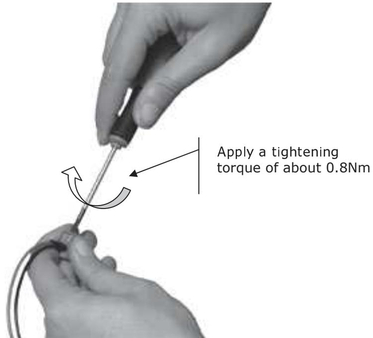
All terminals can tighten correctly cables with section between  $0.1\text{mm}^2$  and  $2.5\text{mm}^2$  (24...14 AWG).
