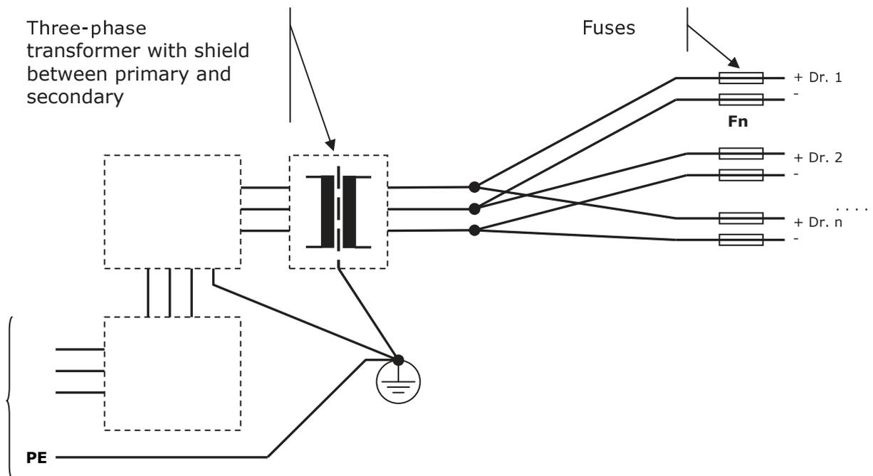
The above scheme includes a three-phase transformer (note the distribution of the drives on the three phases). If necessary it is also possible to use a mono-phase transformer.
