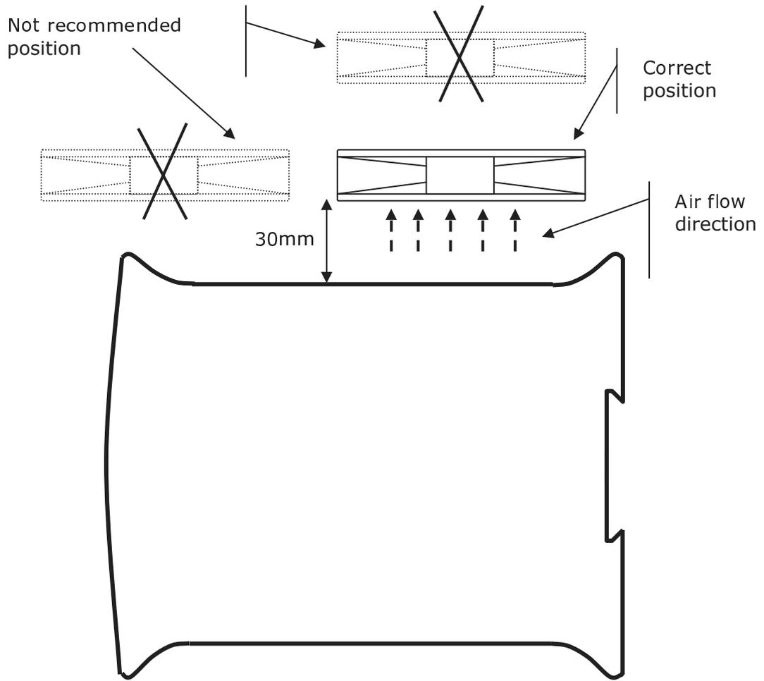
It is important to avoid the drive is covered with powder, dust or other. The buildup of such substances inside the drive could cause the malfunctioning or the breaking of the drive. Filters and necessary solutions must be got ready to avoid these damages to occur.
