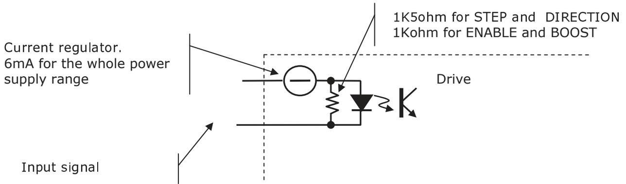
The DS10 drives have on each input a particular current limitation circuit which grants a constant absorption to the varying of the applied voltage. This device allows a wide input power supply range (from 3Vdc up to 28Vdc) without requiring excessive current to the control equipment or external limit resistors.
