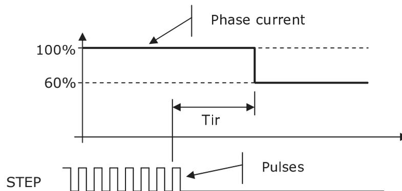
After the last STEP input disable/enable transition the *Tir* time starts to pass, after which the automatic current reduction intervenes reducing the phase current (in the example to the 60% of the nominal value, i.e. of the set configuration value).
