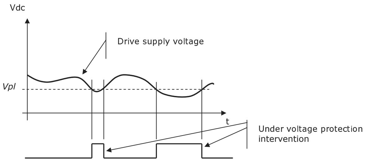
If the supply voltage is very near to the drive functioning limit and sporadically the under voltage alarm intervenes, it is possible, in some cases, to solve the problem reducing the distance between the power supply and the drive, increasing the cables section or placing an electrolytic capacitor near the drive itself (valid only the DC models).
