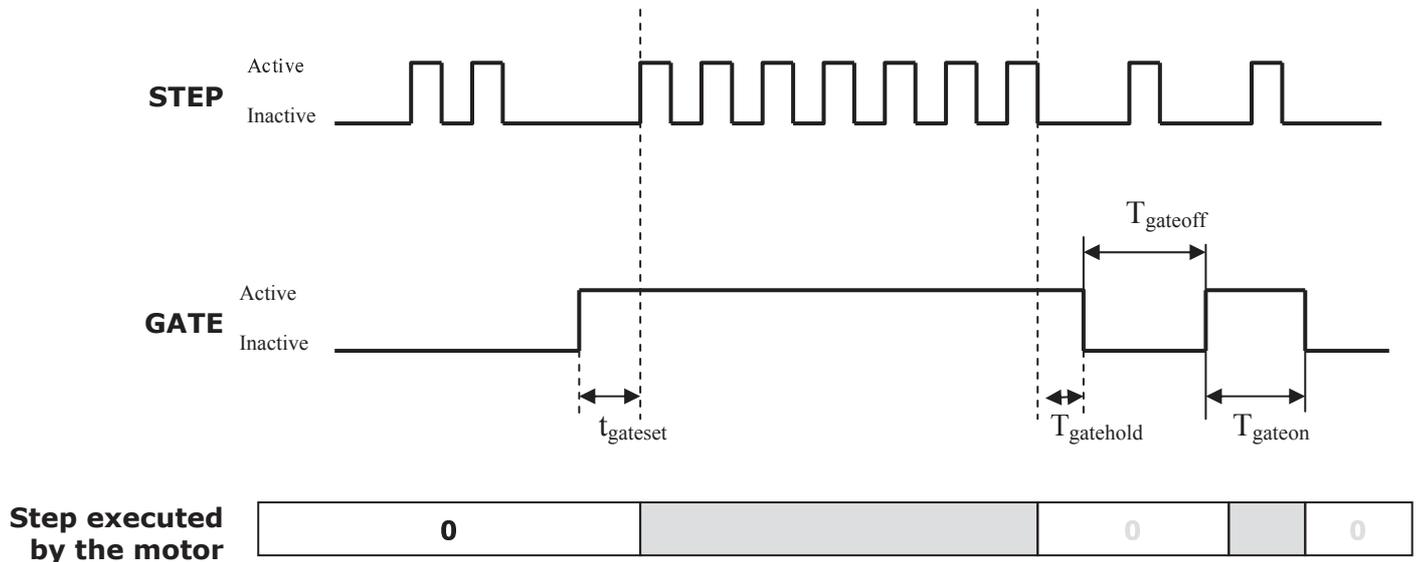
To grant a correct execution of the given commands it is necessary to respect some time relations amongst the signals. In the following table are detailed the limits to be observed.
