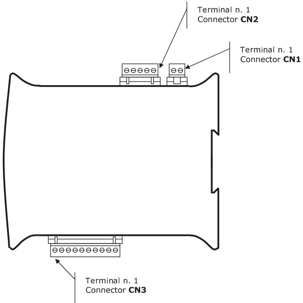
All the terminal blocks do not contain iron and are supplied with mobile truck. The clamping screw is slotted head, sized for screwdriver of 3x0.6mm.
