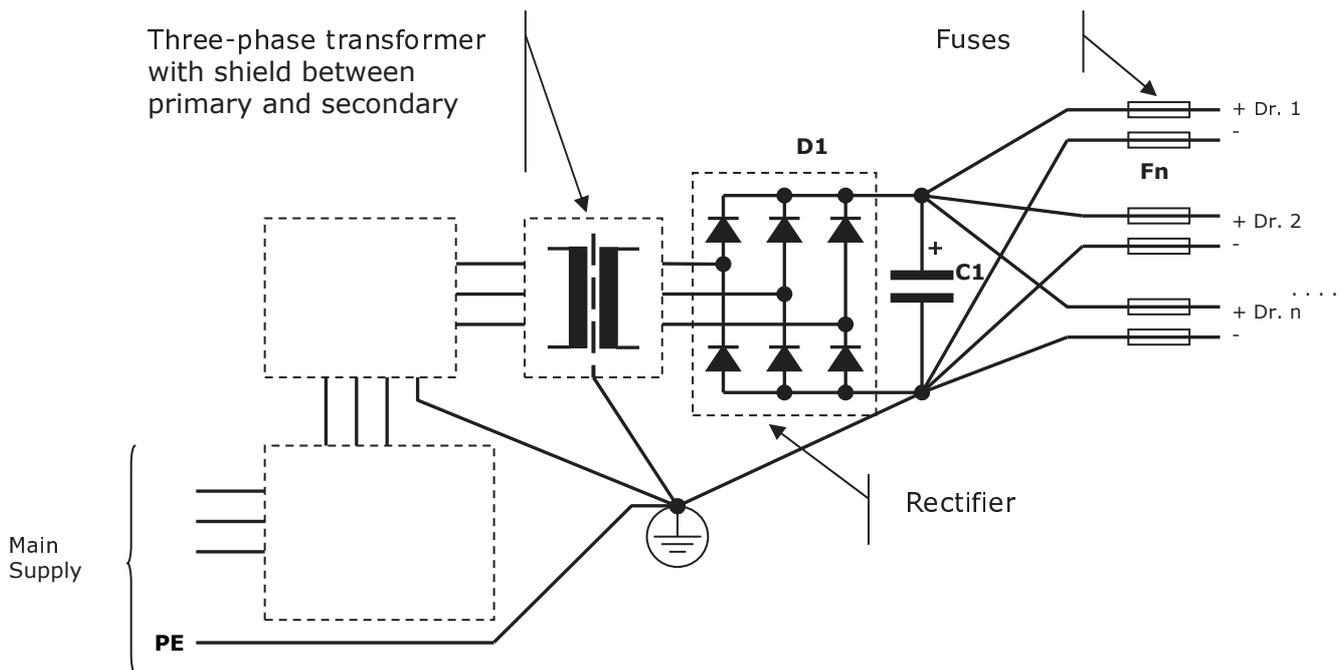
Also note that the wiring must be star-like, where the earth connection of the various components ends in one only point electrically connected to the metal chassis and the earth of the plant.
