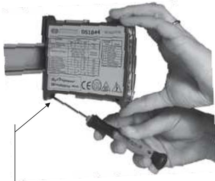
Push the screwdriver slightly downward and pull the drive upward, releasing it from the DIN rail
