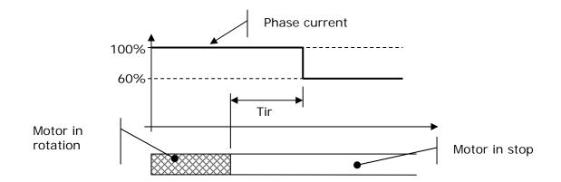
After the stop of the motor the *Tir* time starts to pass, after which the automatic current reduction intervenes reducing the phase current (in the example to the 60% of the nominal value, i.e. of the set value).
