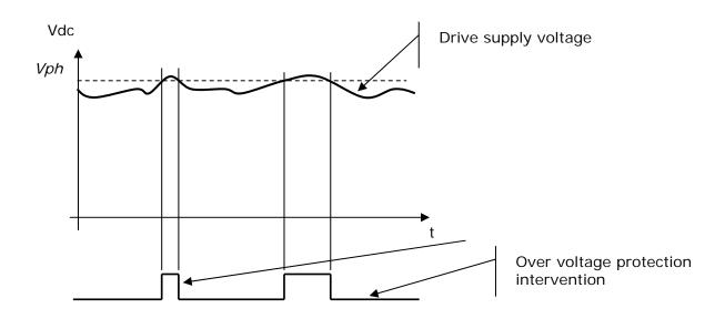
If the supply voltage is very near to the drive functioning limit and the over voltage alarm sporadically intervenes, it is possible in some cases to solve the problem reducing the distance between the power supply and the drive, increasing the cables section or placing an electrolytic capacitor near the drive (valid only for DC models).
