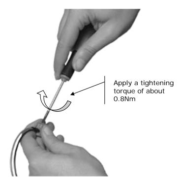
All terminals can tighten correctly cables with section between 0.1 mm<sup>2</sup> and 2.5 mm<sup>2</sup> (24...14 AWG).
