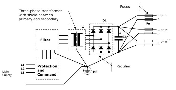
Also note that the wiring must be star-like, where the earth connection of the various components ends in one only point electrically connected to the metal chassis and the earth of the plant.
